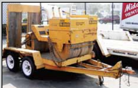
STOW DOUBLE ROLLER ON TRAILER
