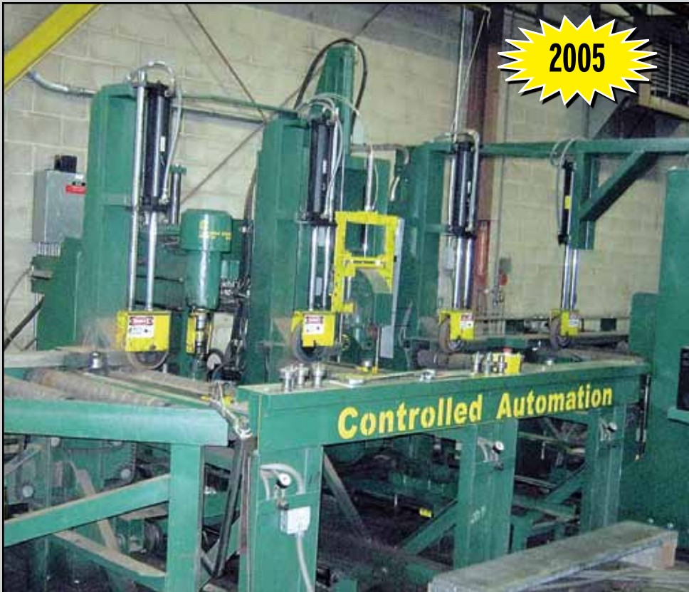
CONTROLLED AUTOMATION CNC BEAM LINE
