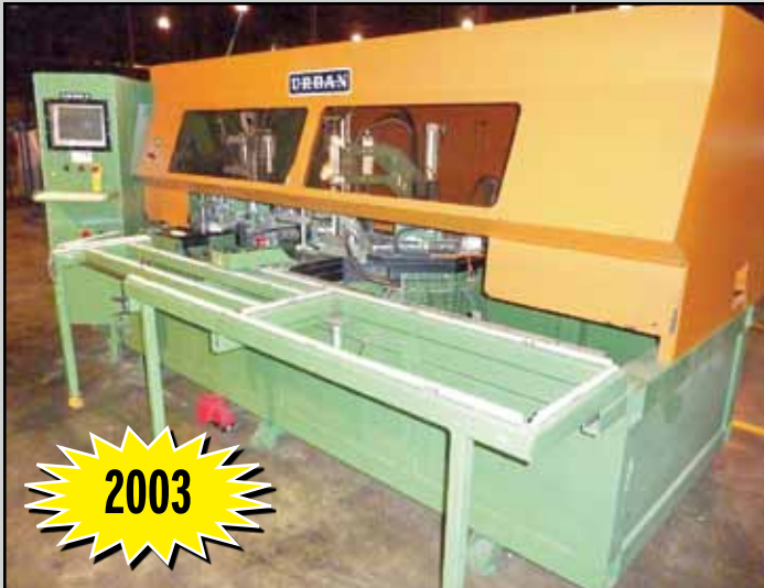
URBAN SV352 CNC WELD SEAM CORNER CLEANER
