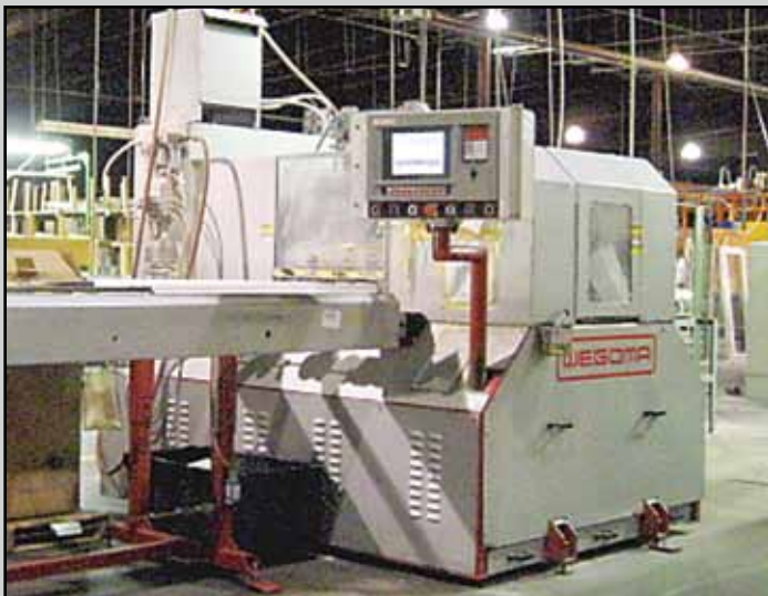
WEGOMA DFM-20 CNC DOUBLE MITER FRAME SAW
