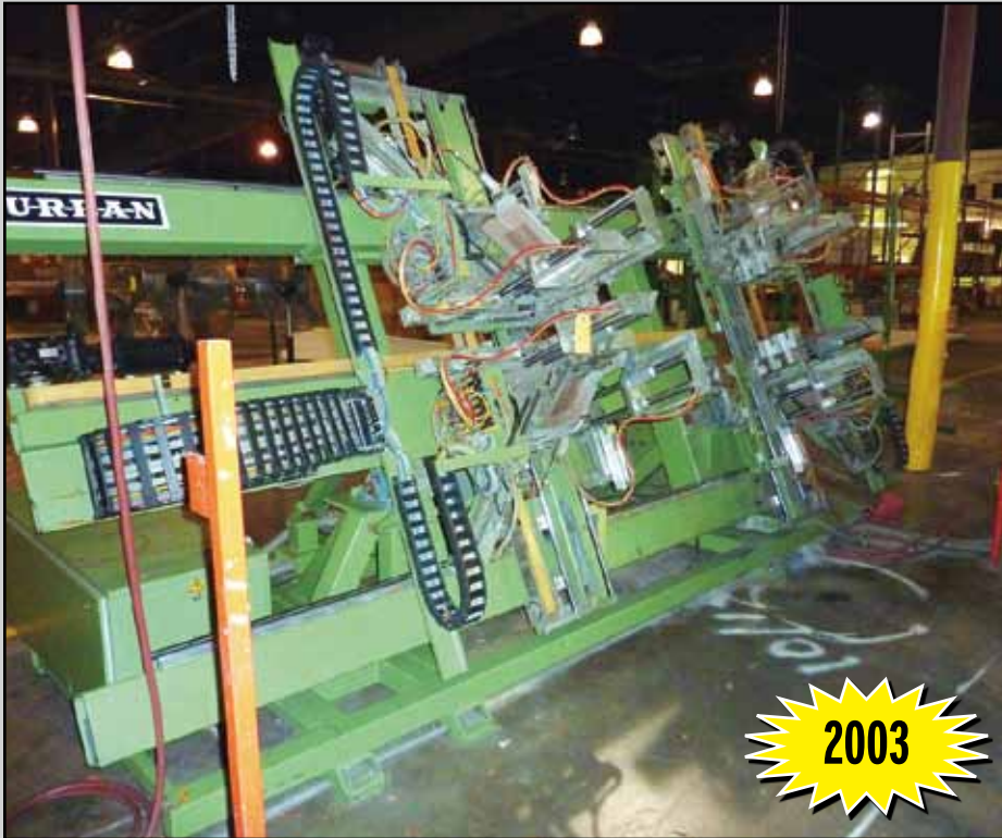
URBAN AKS1400 CNC 4-POINT VERTICAL WELDER
