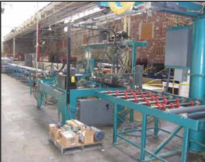
(1 OF 2) KVAL 990 DOOR MACHINES WITH AUTO LOADER & SIX SHOOTER KVAL 950-3 3-Head Semi-Automatic Straight Line Door Jamb Hinge Router.
