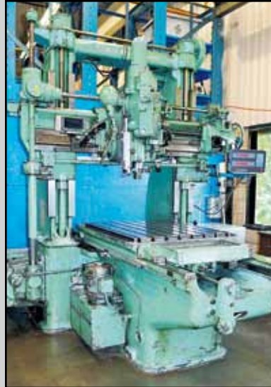
SIP JIG BORER WITH NEW SPINDLE AND DROS
