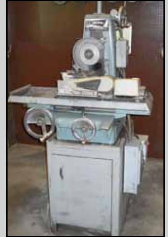
DEDTRU SURFACE GRINDER WITH CENTERLESS GRINDING ATTACHMENT
