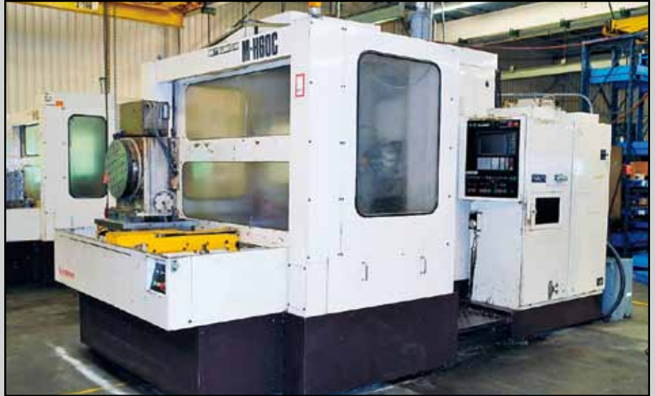
MITSUBISHI M-H60C CNC HORIZONTAL MACHINING CENTER WITH 4TH AXIS ROTARY TABLE
