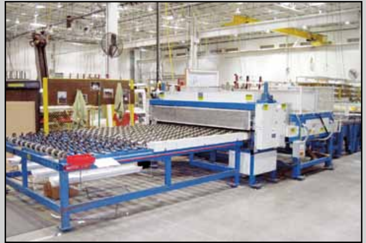
GED CURING OVEN
