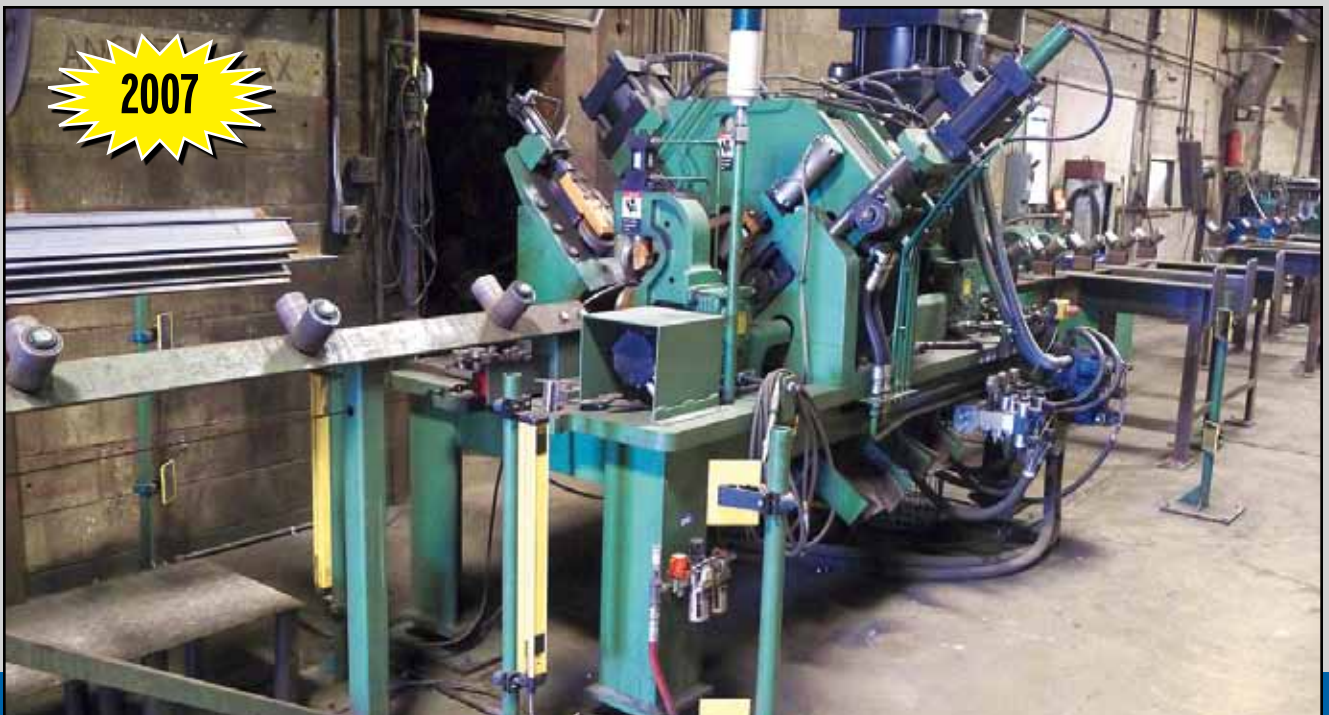
PEDDINGHAUS ANGLEMASTER 643 CNC ANGLE CUTTING AND PUNCHING LINE
