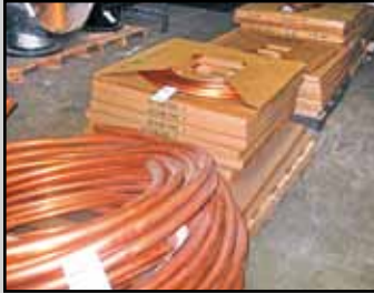
COILED COPPER PIPE
