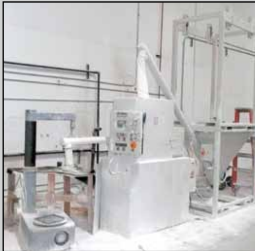
(1 OF 3) GRUBER BATCH MASTER RESIN SPRAYER WITH FEEDER BIN
