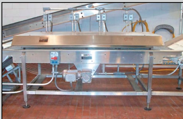
DRYING CONVEYOR (SEEDER)
