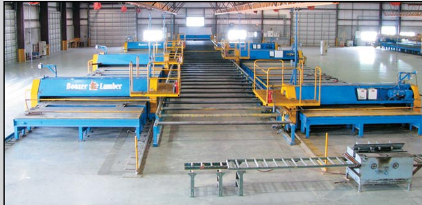
VIEW OF (2 OF 4) MITEK ROOF TRUSS LINES
