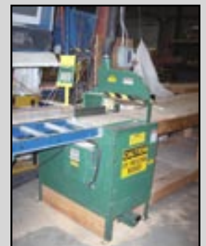
(1 OF 2) UP-ACTING CUTOFF SAWS, WITH PLC CONTROLS
